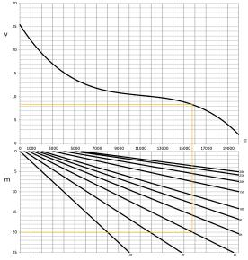
v=speed [km/h], m=incline [%], F=drawbar pull [N]
