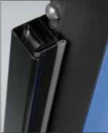
The wear-resistant Lexan guides of the wind retention system are rigid enough to keep tension on the curtain, yet flexible enough to break away when there is an impact.
